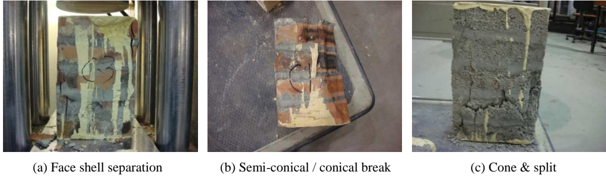
Figure 1. Different failure modes of masonry prisms
