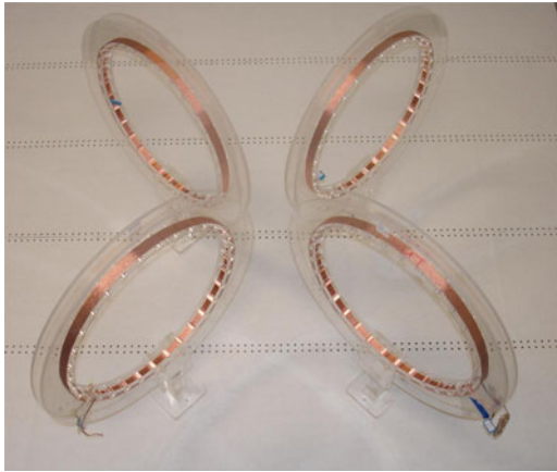
Fig. 15. Circular four-resonator system.
