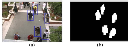
Fig. 2. Examples of training images. (a) Training persons are annotated with a rectangular bounding box. (b) Foreground region for training persons.
