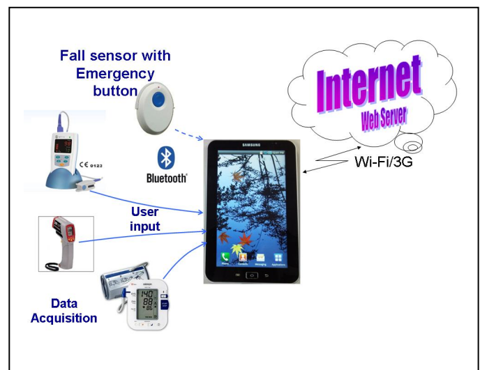
Figure 1. Android tablet with App to receive emergency signal or health data for uploading
