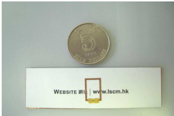
Fig. 7. The fabricated prototype of the loop-fed double patches antenna, the total dimension is 80 mm \times 25 mm \times 3.5 mm.
