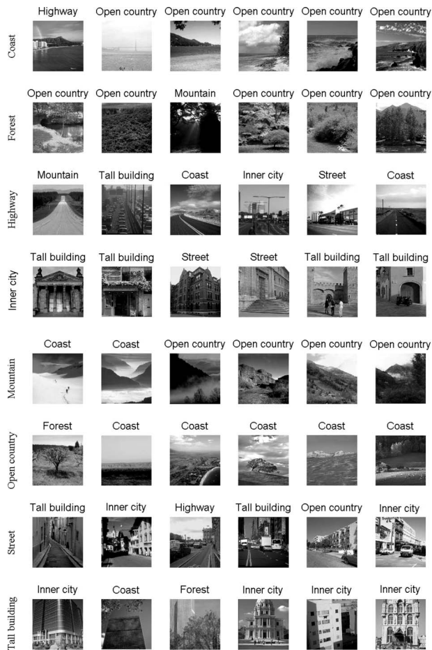
Fig. 13 Misclassified samples. (Words above the images are the labels predicted by the classifier, and the word on the left of each row is the true label of the images in that row.)
