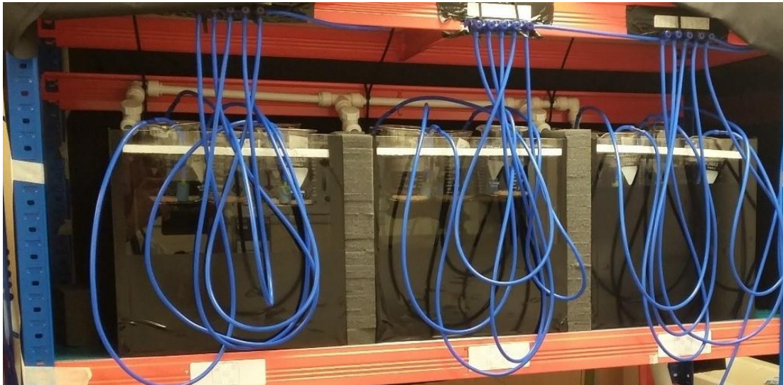
Figure 66 The embryo rearing system at the Hastings laboratory in use incubating Salmo trutta embryos. The front black out curtain is lifted to show three semi-blacked out aquaria with airlines running into beakers suspended into chilled re-circulating water
