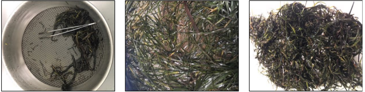
Figure 4.2: Above-ground biomass being washed free of soil and under running water, using a 1mm sieve.
