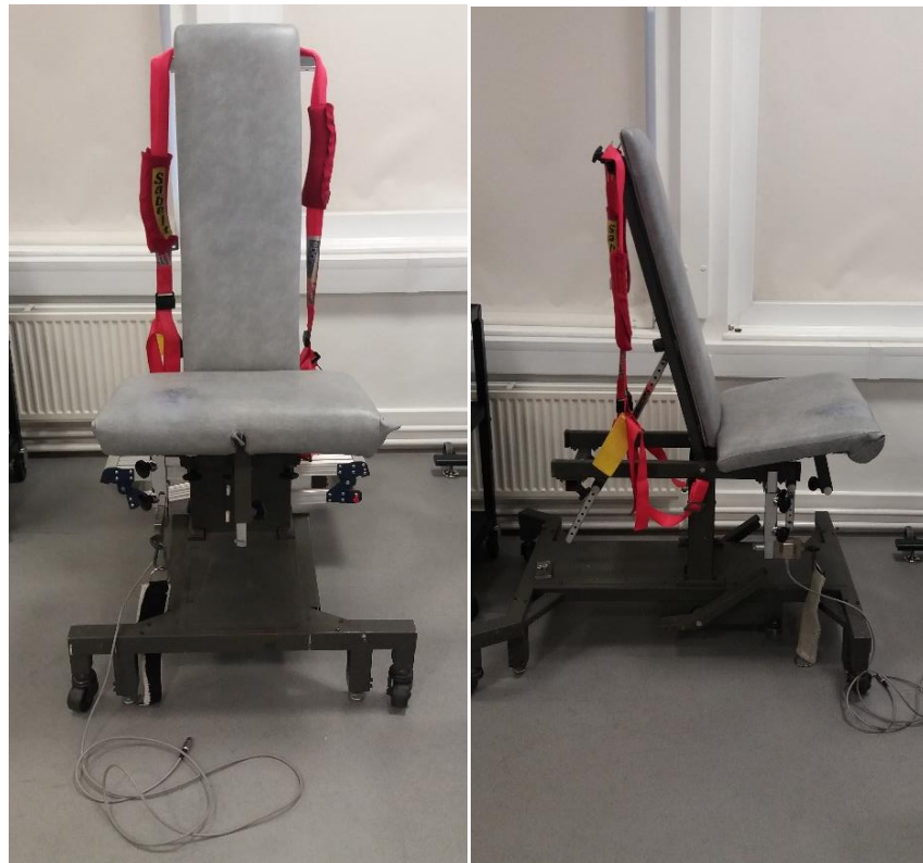
Figure 3.3. The custom-built isometric rig at the Welkin Laboratories, University of Brighton
