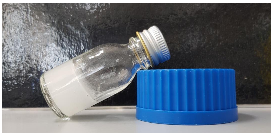
Figure 4.25 - Image of an alginate hydrogel, formed within a 15 ml bijoux bottle, cross-linked using the \text{CaCO}_3 -GDL system of internal liberation of \text{Ca}^{2+} ions. Final concentrations of the hydrogel formulation were as follows; 1.5 % alginate, 1 % GDL, and 1 % \text{CaCO}_3 .
