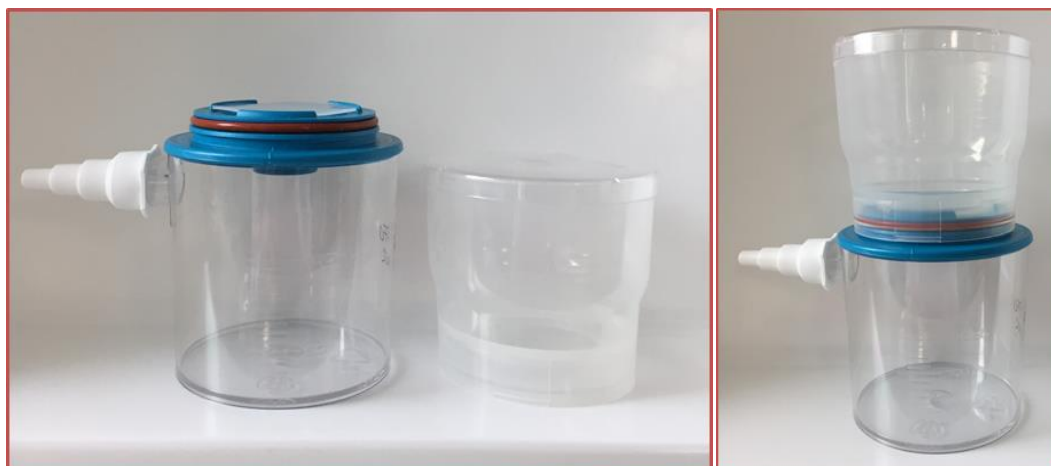
Figure 5.2 - Images of bacterial filter units utilised for bacteriophage adsorption and dissociation studies.
