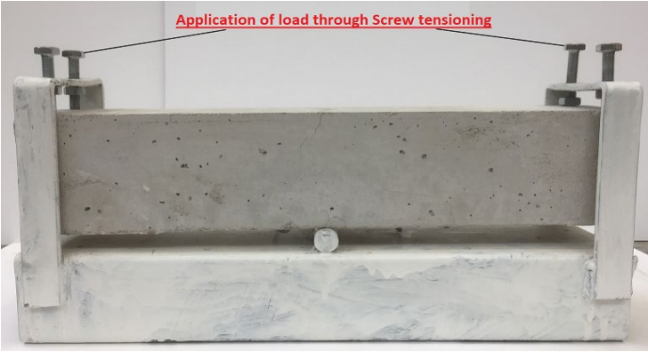
a: Flexural method for cracking in the prism samples
