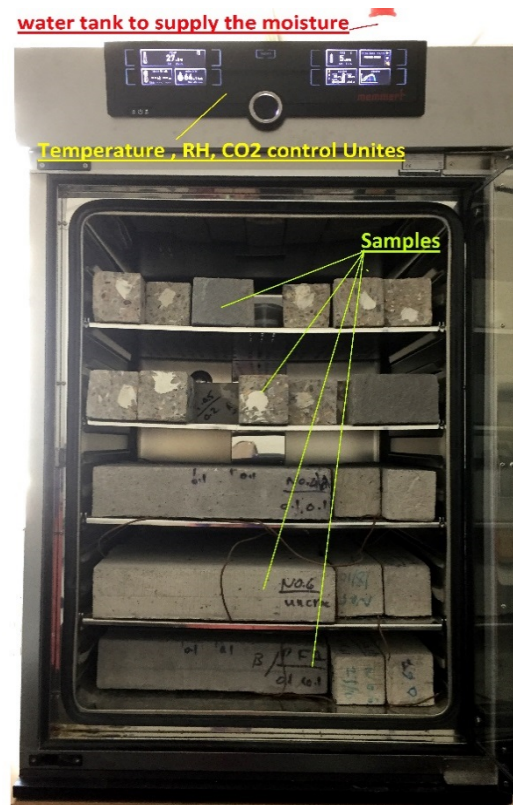
Figure 3.13: The exposure conditions CO 2 concentration, temperature and relative humidity was considered in the incubator
