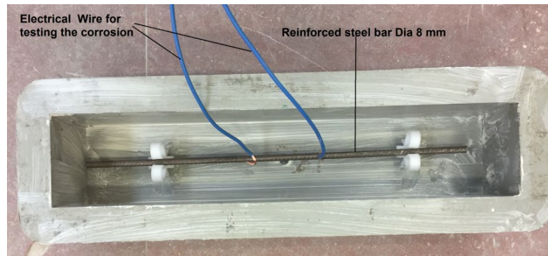
Figure 3.10: Mould with a steel bar for casting reinforced concrete prism
