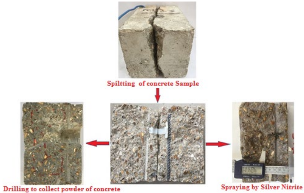
Figure 3.25: The steps of collecting powder from concrete to measure chloride concentration in concrete specimen
