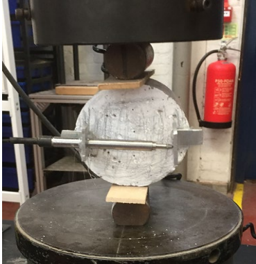
c: The crack by splitting test
