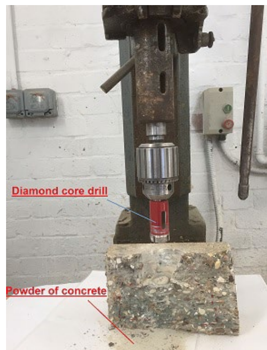
Figure 3.26: Dry drilling of the concrete sample to collect the powder of concrete
