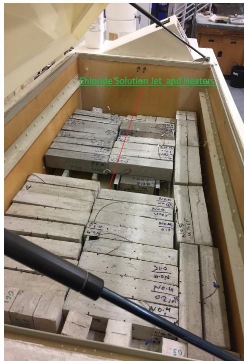
Figure 3.15: CCT Chamber for accelerating the chloride penetration and corrosion
