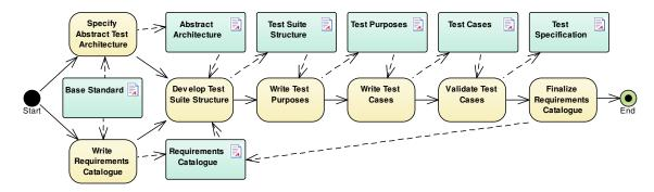
Figure 4.4: Development of a Test Specification (adapted from [22, Section 8])
