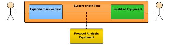
Figure 4.3: Interoperability Testing with Conformance Analysis (adapted from [22, Section 4.3])
