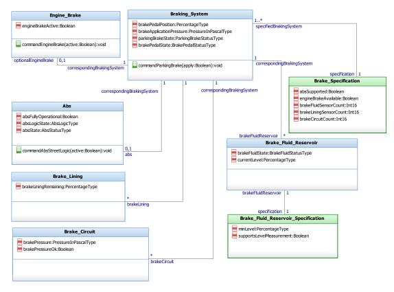
Figure 5.1: NGVA Brakes PIM Class Diagram
