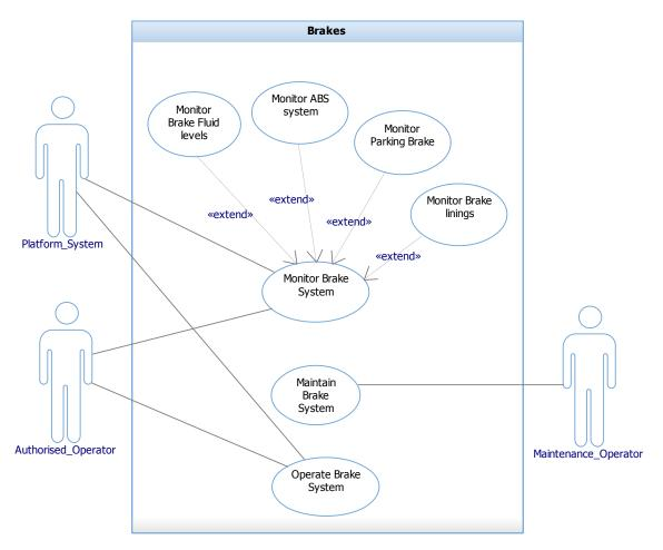
Figure 5.2: NGVA Brakes PIM Use Case Diagram
