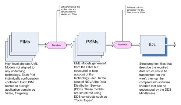
Figure 2.4: MDA Approach for NGVA DM Modules according to [4]
