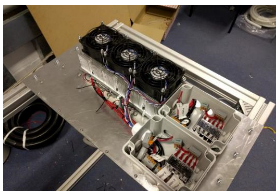
Figure 49: Position of the cooling stage assembly in the rack
