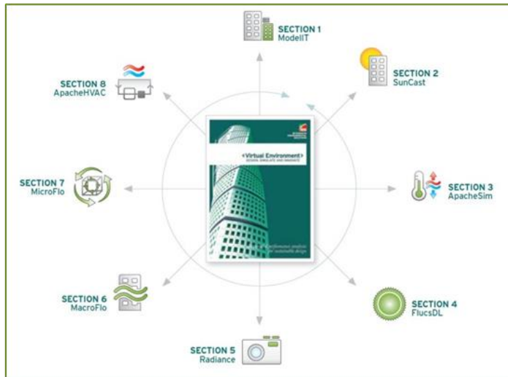
Figure 4.5 Modules integrated in IES-VE
