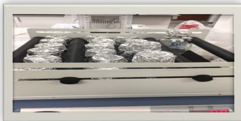
Figure 3.6 Orbital shaking of samples.
