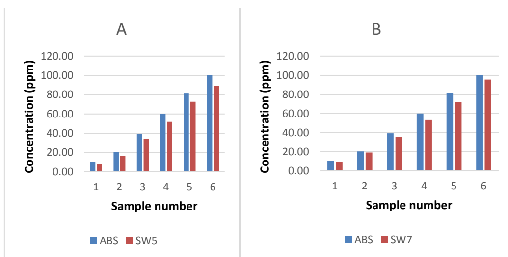
Figure 6.4 Adsorption of Phenol using (a) Soft-wood 550 and (b) 700. (ABS = absorbance prior to experiment, while ADS = after adsorption experiment). The y-axis shows Phenol concentrations in parts per million. The x-axis shows sample numbers.
