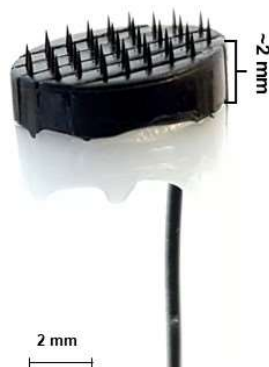
Figure 4.6. Digital image of an optimised MNA fabricated using the nanocomposite material. The electrical contact was sealed with PCL.
