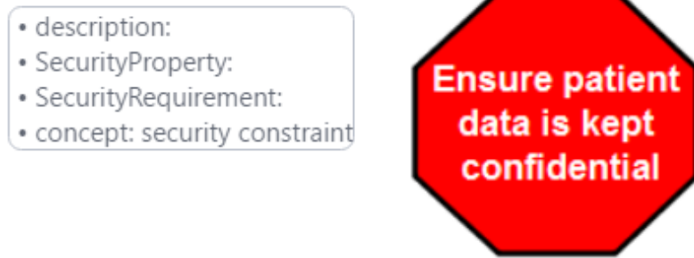
Figure 3.32: A security constraint visualised as a red octagon with a black outline.
