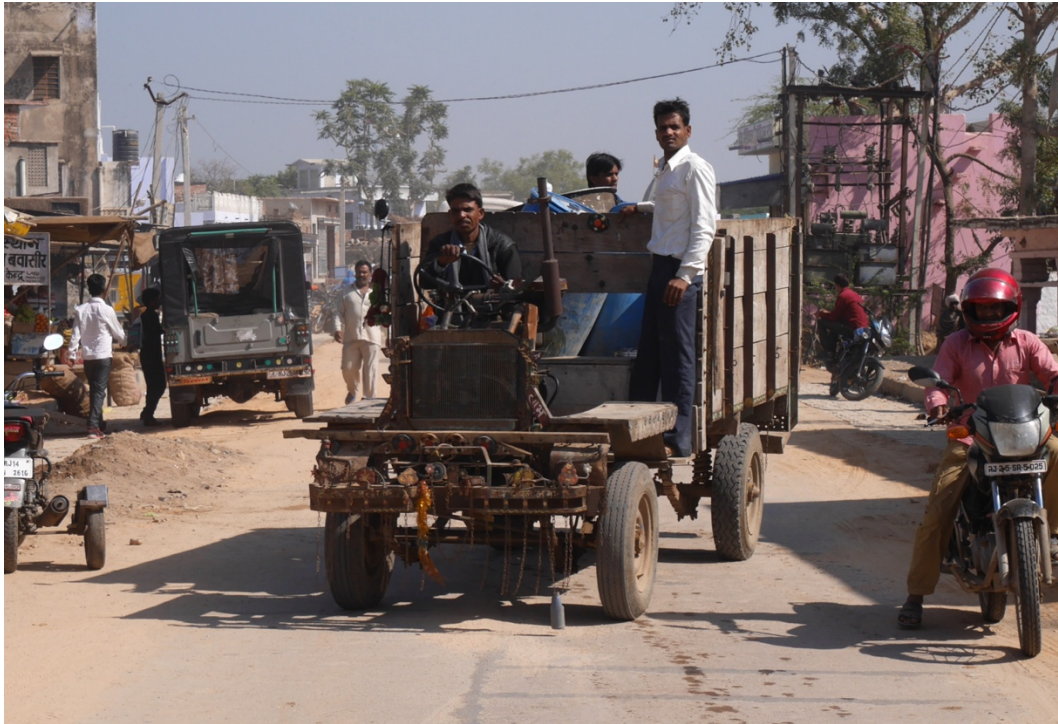
Figure 1. A jugaad truck in a market town in Sawai Madhopur district, Rajasthan (Photo: Willy Logan)
