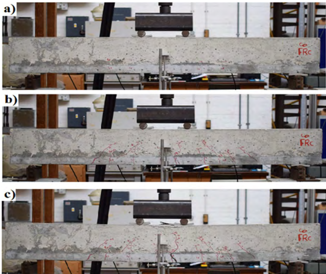
Figure 8.9 Crack pattern of beams repaired using FRC composites a) during first crack formation, b) before reaching the ultimate load and c) after failure.
