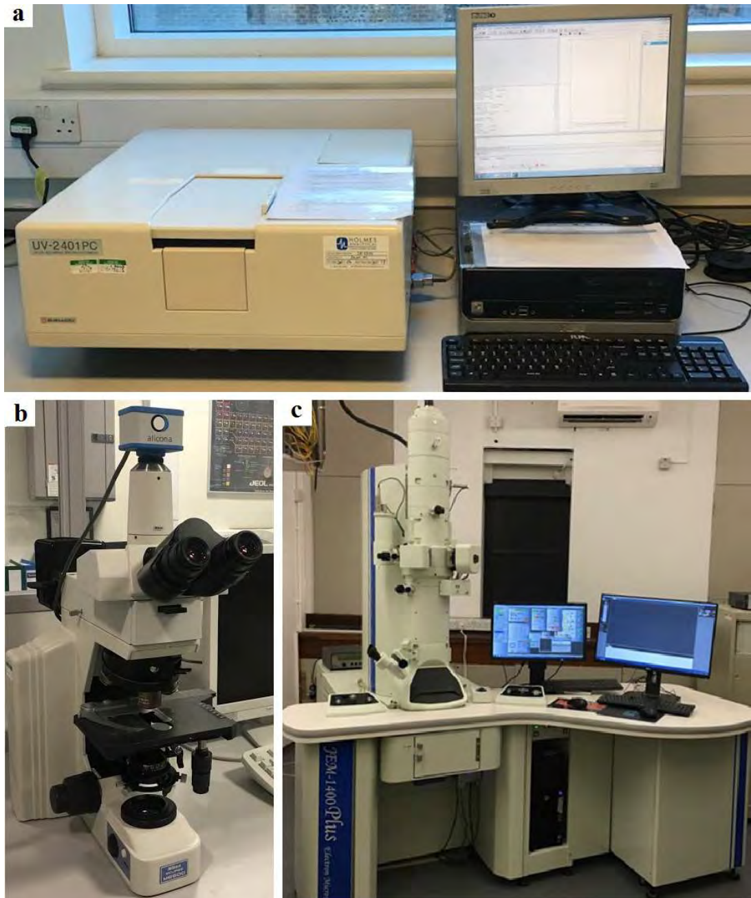
Figure 3.4 a) Ultraviolet-visible spectroscopy model (UV-2401PC), b) polarization optical microscope (Amplival Pol. D, Carl Zeiss, Tena, German), and c), Transmission electron microscope (TEM).
