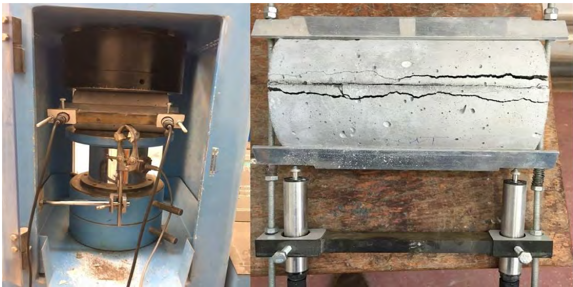
Figure 6.5 Test set-up for cylinders under uniaxial load.
