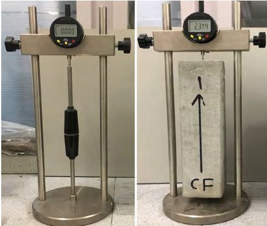
Figure 3.12 Set-up for evaluating free drying shrinkage.
