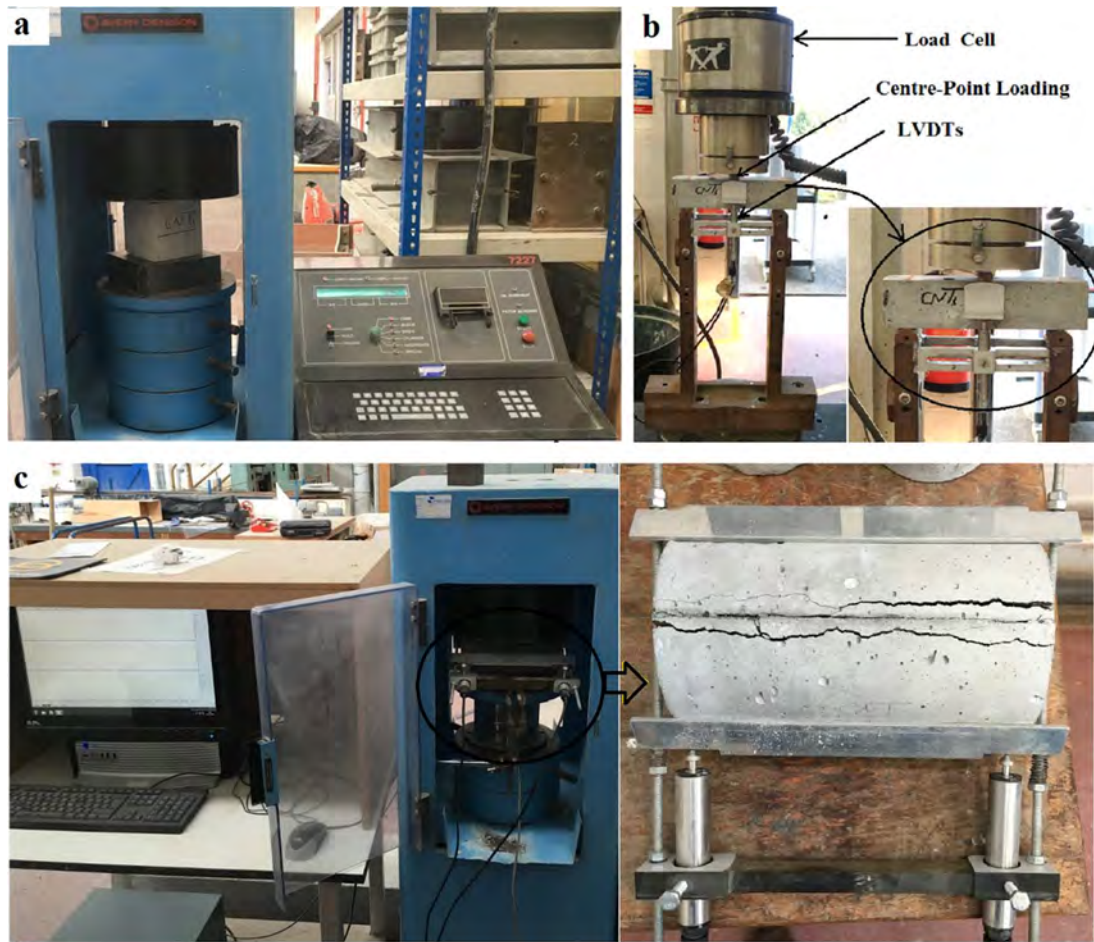
Figure 3.8 Test set-up of a) compressive strength, b) flexural strength, and c) splitting tensile strength tests.
