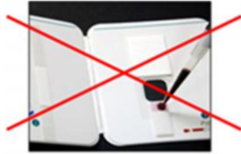
DO NOT add blood directly to the pink portion of the sample pad
