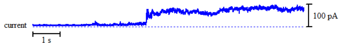
Figure A2 - 3: Above: bilayer activity of 8 with Na + ions upon the addition of 150μl stock solution of 8 in DMSO. Right: histogram displaying the average currents for the above trace: peak 1 = 8.7040 ± 0.0589 pA and peak 2 = 80.1100 ± 0.3392 pA.
