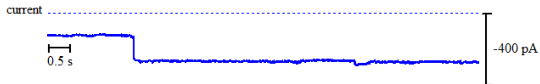
Figure A2 - 27: Above: bilayer activity of 8 with Na + ions upon the addition of 175μl stock solution of 8 in DMSO. Right: histogram displaying the average currents for the above trace: peak 1 = -268.4 ± 0.0413 pA and peak 2 = -125.0 ± 0.0591 pA.
