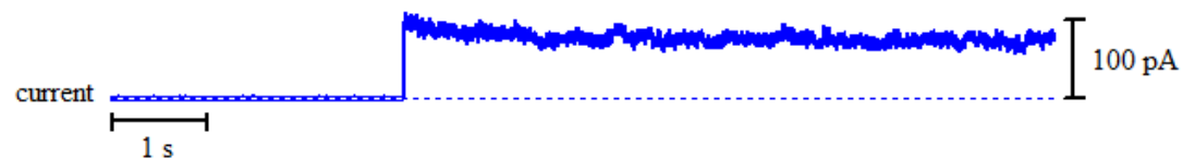
Figure A2 - 143: Above: bilayer activity of 14 with Na + ions upon the addition of 50 \mu l stock solution of 14 in DMSO. Right: histogram displaying the average currents for the above trace: peak 1 = 0.4345 \pm 0.0070 pA and peak 2 = 77.52 \pm 0.0996 pA.
