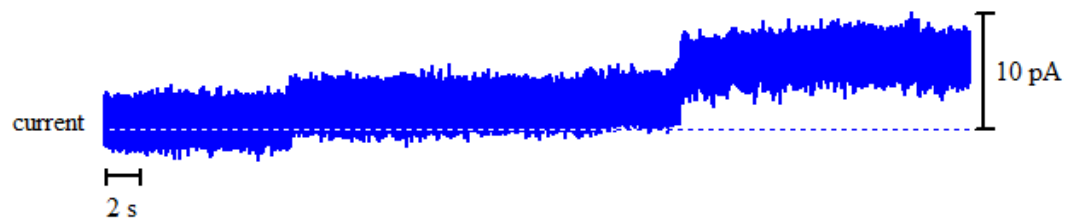
Figure A2 - 122: Above: bilayer activity of 13 with Na + ions upon the addition of 75 \mu l stock solution of 13 in DMSO. Right: histogram displaying the average currents for the above trace: peak 1 = 1.776 \pm 0.0160 pA and peak 2 = 6.249 \pm 0.0267 pA.
