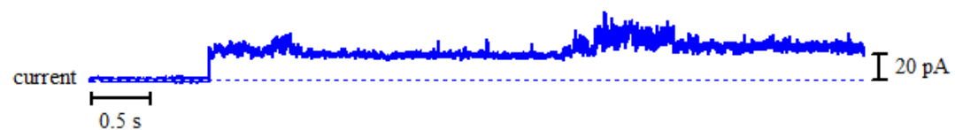
92 Figure A2 - 12: Above: bilayer activity of 8 with K^+ ions upon the addition of 175 \mu l stock solution of 8 in DMSO. Right: histogram displaying the average currents for the above trace: peak 1 = 0.686 \pm 0.0274 pA, peak 2 = 19.4 \pm 0.0317 pA and peak 3 = 25.6 \pm 0.1118 pA.
