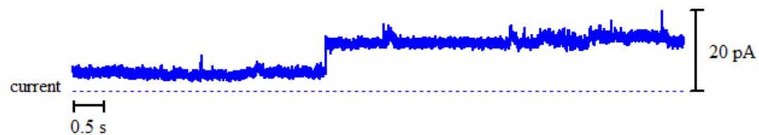
Figure A2 – 94: Above: bilayer activity of 11 with Na + ions upon the addition of 175 \mu l stock solution of 11 in DMSO. Right: histogram displaying the average currents for the above trace: peak 1 = 4.445 \pm 0.0048 pA, peak 2 = 12.03 \pm 0.0109 pA and peak 3 = 13.58 \pm 0.0474 pA.
