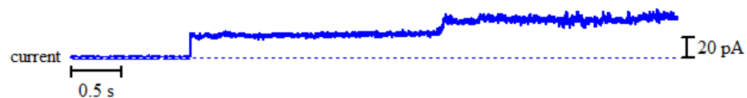
Figure A2 - 166: Above: bilayer activity of 15 with K^+ ions upon the addition of 250 \mu l stock solution of 15 in DMSO. Right: histogram displaying the average currents for the above trace: peak 1 = 0.6839 \pm 0.0068 pA, peak 2 = 23.22 \pm 0.0114 pA and peak 3 = 38.18 \pm 0.0416 pA .
