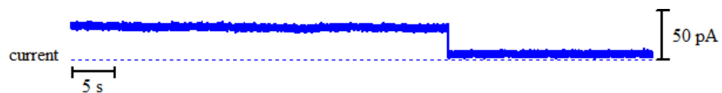
Figure A2 - 54: Above: bilayer activity of 8 with Rb + ions upon the addition of 175 μl stock solution of 8 in DMSO. Right: histogram displaying the average currents for the above trace: peak 1 = 6.311 ± 0.0050 pA and peak 2 = 32.94 ± 0.0102 pA.
