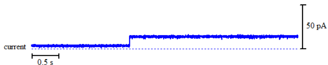
Figure A2 - 6: Above: bilayer activity of 8 with Na + ions upon the addition of 200 \mu l stock solution of 8 in DMSO. Right: histogram displaying the average currents for the above trace: peak 1 = 3.642 \pm 0.008 pA and peak 2 = 14.14 \pm 0.0084 pA.
