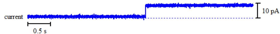
Figure A2 - 157: Above: bilayer activity of 14 with Na + ions upon the addition of 125μl stock solution of 14 in DMSO. Right: histogram displaying the average currents for the above trace: peak 1 = 1.069 ± 0.0044 pA and peak 2 = 8.796 ± 0.0050 pA.
