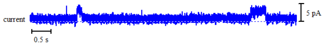
Figure A2 - 44: Above: bilayer activity of 8 with K^+ ions upon the addition of 200 \mu l stock solution of 8 in DMSO. Right: histogram displaying the average currents for the above trace: peak 1 = 0.8565 \pm 0.0107 pA and peak 2 = 3.035 \pm 0.129 pA.
