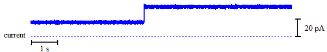
Figure A2 - 194: Above: bilayer activity of 18 with Na + ions upon the addition of 75μl stock solution of 18 in DMSO. Right: histogram displaying the average currents for the above trace: peak 1 = 16.78 \pm 0.0080 pA and peak 2 = 34.79 \pm 0.0089 pA.
