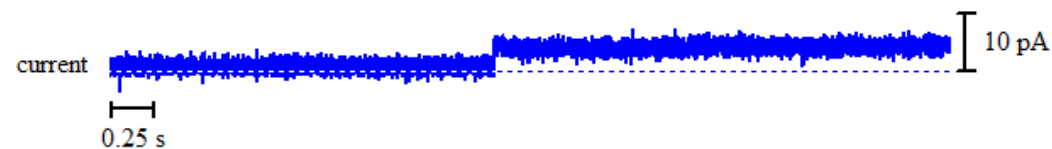
Figure A2 - 78: Above: bilayer activity of 10 with Na + ions upon the addition of 200 μl stock solution of 10 in DMSO. Right: histogram displaying the average currents for the above trace: peak 1 = 0.9736 \pm 0.0106 pA and peak 2 = 4.382 \pm 0.0090 pA.
