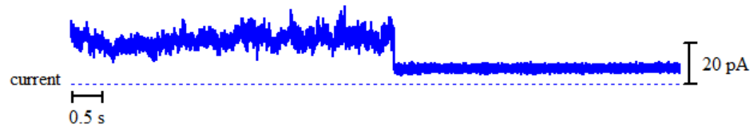
Figure A2 - 161: Above: bilayer activity of 15 with Na + ions upon the addition of 200 \mu l stock solution of 15 in DMSO. Right: histogram displaying the average currents for the above trace: peak 1 = 8.243 \pm 0.0050 pA and peak 2 = 22.24 \pm 0.0318 pA.
