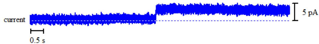
Figure A2 - 50: Above: bilayer activity of 8 with Li + ions upon the addition of 50 \mu l stock solution of 8 in DMSO. Right: histogram displaying the average currents for the above trace: peak 1 = 0.4493 \pm 0.0117 pA and peak 2 = 3.316 \pm 0.0134 pA.
