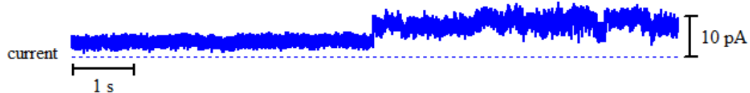
Figure A2 - 192: Above: bilayer activity of 18 with Na + ions upon the addition of 100 \mu l stock solution of 18 in DMSO. Right: histogram displaying the average currents for the above trace: peak 1 = 3.927 \pm 0.0079 pA and peak 2 = 8.524 \pm 0.0196 pA.
