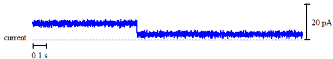
Figure A2 - 123: Above: bilayer activity of 13 with Na + ions upon the addition of 100 \mu l stock solution of 13 in DMSO. Right: histogram displaying the average currents for the above trace: peak 1 = 3.37 \pm 0.0059 pA and peak 2 = 9.311 \pm 0.0427 pA.
