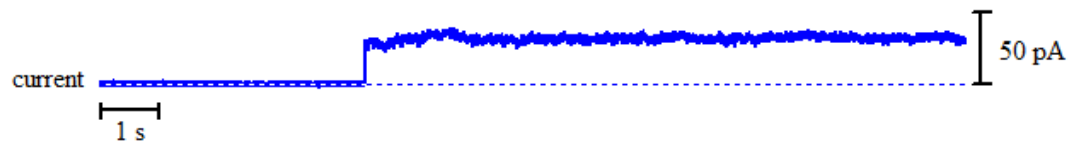
Figure A2 - 25: Above: bilayer activity of 8 with Na + ions upon the addition of 100μl stock solution of 8 in DMSO. Right: histogram displaying the average currents for the above trace: peak 1 = 0.5715 ± 0.0047 pA and peak 2 = 31.83 ± 0.0230 pA.
