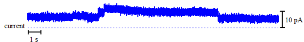
Figure A2 - 96: Above: bilayer activity of 11 with Na + ions upon the addition of 175μl stock solution of 11 in DMSO. Right: histogram displaying the average currents for the above trace: peak 1 = 6.342 ± 0.0204 pA and peak 2 = 10.06 ± 0.0265 pA.
