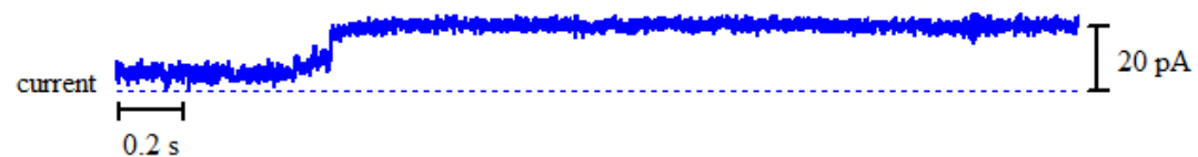
Figure A2 - 141: Above: bilayer activity of 14 with Na + ions upon the addition of 75μl stock solution of 14 in DMSO. Right: histogram displaying the average currents for the above trace: peak 1 = 5.813 ± 0.0756 pA and peak 2 = 20.68 ± 0.0109 pA.
