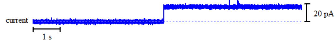
Figure A2 - 142: Above: bilayer activity of 14 with Na + ions upon the addition of 75μl stock solution of 14 in DMSO. Right: histogram displaying the average currents for the above trace: peak 1 = 0.3026 ± 0.0086 pA and peak 2 = 17.25 ± 0.0095 pA.
