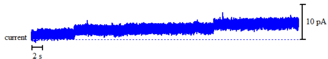
Figure A2 - 91: Above: bilayer activity of 11 with Na + ions upon the addition of 100μl stock solution of 11 in DMSO. Right: histogram displaying the average currents for the above trace: peak 1 = 1.611 ± 0.0740 pA, peak 2 = 3.054 ± 0.0347 pA and peak 3 = 4.439 ± 0.2179 pA.
