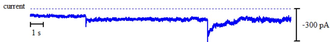
Figure A2 - 24: Above: bilayer activity of 8 with Na + ions upon the addition of 150μl stock solution of 8 in DMSO. Right: histogram displaying the average currents for the above trace: peak 1 = -131.3 \pm 0.9404 pA, peak 2 = -96.84 \pm 0.0781 pA and peak 3 = -64.66 \pm 0.1414 pA.
