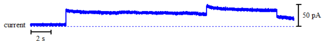
Figure A2 - 52: Above: bilayer activity of 8 with Rb + ions upon the addition of 175 μl stock solution of 8 in DMSO. Right: histogram displaying the average currents for the above trace: peak 1 = 4.585 \pm 0.0056 pA, peak 2 = 21.07 \pm 0.1370 pA, peak 3 = 31.95 \pm 0.0202 pA and peak 4 = 38.91 \pm 0.0653 pA.
