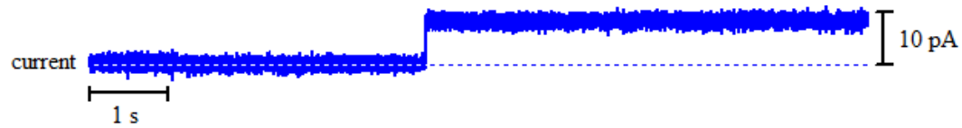
Figure A2 - 184: Above: bilayer activity of 17 with Na + ions upon the addition of 250 μl stock solution of 17 in DMSO. Right: histogram displaying the average currents for the above trace: peak 1 = 0.3271 ± 0.0072 pA and peak 2 = 8.563 ± 0.0073 pA.
