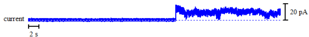
Figure A2 - 23: Above: bilayer activity of 8 with Na + ions upon the addition of 125μl stock solution of 8 in DMSO. Right: histogram displaying the average currents for the above trace: peak 1 = 0.5275 \pm 0.0043 pA and peak 2 = 9.956 \pm 0.0533 pA.
