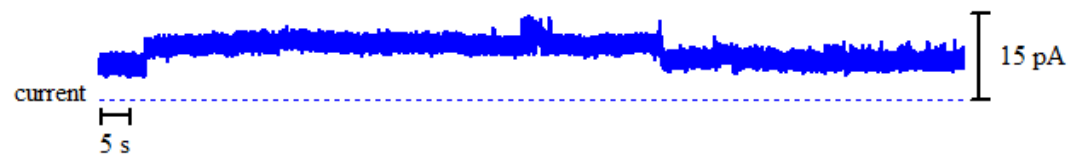
Figure A2 - 92: Above: bilayer activity of 11 with Na + ions upon the addition of 100 \mu l stock solution of 11 in DMSO. Right: histogram displaying the average currents for the above trace: peak 1 = 6.784 \pm 0.0581 pA and peak 2 = 9.733 \pm 0.0083 pA.
