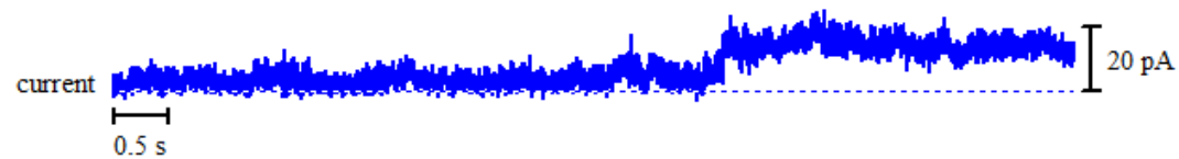
Figure A2 - 164: Above: bilayer activity of 15 with K^+ ions upon the addition of 75 \mu l stock solution of 15 in DMSO. Right: histogram displaying the average currents for the above trace: peak 1 = 3.536 \pm 0.0260 pA and peak 2 = 14.21 \pm 0.0598 pA.
