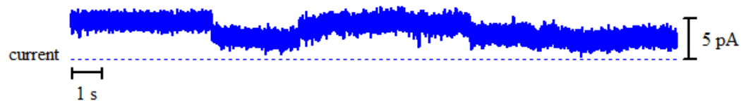
Figure A2 - 93: Above: bilayer activity of 11 with Na + ions upon the addition of 150 \mu l stock solution of 11 in DMSO. Right: histogram displaying the average currents for the above trace: peak 1 = 2.862 \pm 0.0144 pA and peak 2 = 4.603 \pm 0.0118 pA.
