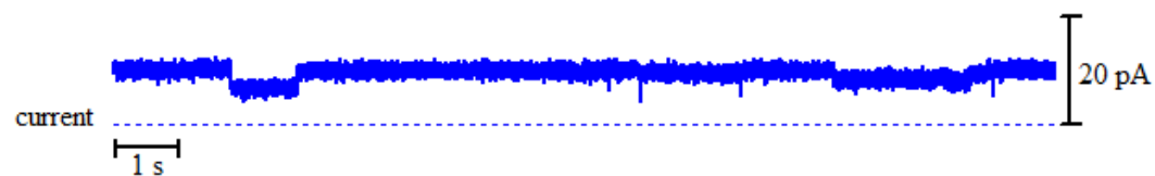
Figure A2 - 20: Above: bilayer activity of 8 with Na + ions upon the addition of 150 μl stock solution of 8 in DMSO. Right: histogram displaying the average currents for the above trace: peak 1 = 6.67 ± 0.0173 pA and peak 2 = 10.16 ± 0.0101 pA.
