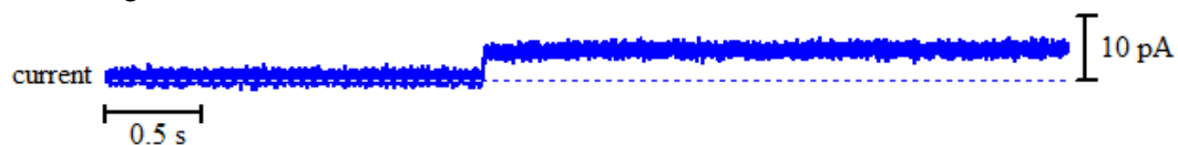
Figure A2 - 57: Above: bilayer activity of 8 with Cs + ions upon the addition of 25 μl stock solution of 8 in DMSO. Right: histogram displaying the average currents for the above trace: peak 1 = 0.601 \pm 0.0135 pA and peak 2 = 4.875 \pm 0.0124 pA.
