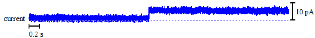
Figure A2 - 84: Above: bilayer activity of 11 with Na + ions upon the addition of 75 \mu l stock solution of 11 in DMSO. Right: histogram displaying the average currents for the above trace: peak 1 = 1.173 \pm 0.0156 pA and peak 2 = 5.601 \pm 0.0137 pA.
