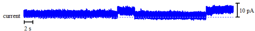
Figure A2 - 86: Above: bilayer activity of 11 with Na + ions upon the addition of 150 μl stock solution of 11 in DMSO. Right: histogram displaying the average currents for the above trace: peak 1 = 2.018 ± 0.0229 pA and peak 2 = 5.162 ± 0.0919 pA.
