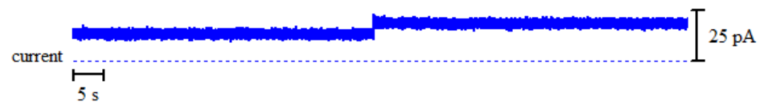
Figure A2 - 97: Above: bilayer activity of 11 with Na + ions upon the addition of 200μl stock solution of 11 in DMSO. Right: histogram displaying the average currents for the above trace: peak 1 = 13.87 ± 0.0077 pA and peak 2 = 19.03 ± 0.0071 pA.
