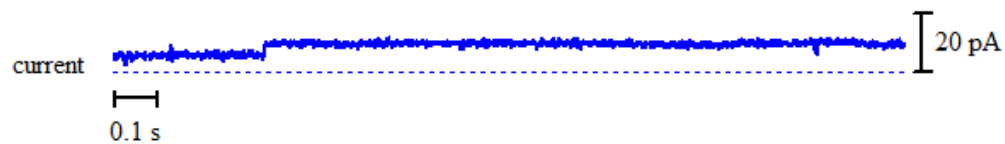
Figure A2 - 18: Above: bilayer activity of 8 with Na + ions upon the addition of 150μl stock solution of 8 in DMSO. Right: histogram displaying the average currents for the above trace: peak 1 = 5.947 ± 0.0396 pA and peak 2 = 9.963 ± 0.0108 pA.
