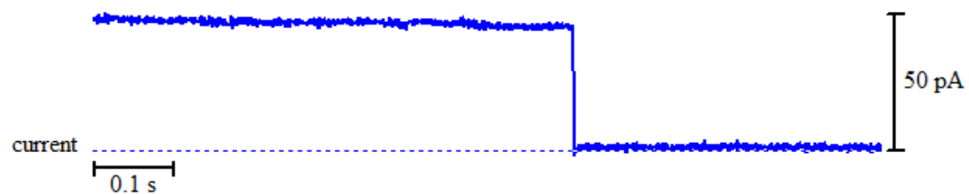
Figure A2 - 34: Above: bilayer activity of 8 with Na + ions upon the addition of 50 \mu l stock solution of 8 in DMSO. Right: histogram displaying the average currents for the above trace: peak 1 = 46.77 \pm 0.0176 pA and peak 2 = 1.063 \pm 0.0038 pA.
