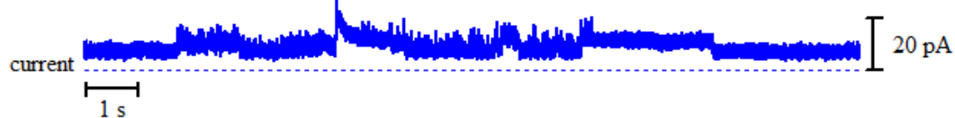
Figure A2 - 89: Above: bilayer activity of 11 with Na + ions upon the addition of 200μl stock solution of 11 in DMSO. Right: histogram displaying the average currents for the above trace: peak 1 = 7.757 ± 0.0147 pA and peak 2 = 11.62 ± 0.0427 pA.
