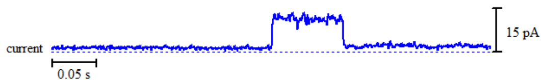
Figure A2 - 124: Above: bilayer activity of 13 with \text{Na}^+ ions upon the addition of 200 \mu\text{l} stock solution of 13 in DMSO. Right: histogram displaying the average currents for the above trace: peak 1 = 1.729 \pm 0.0118 pA and peak 2 = 11.3 \pm 0.2743 pA.
