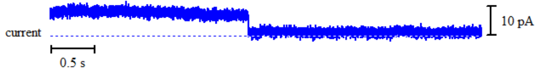
Figure A2 - 85: Above: bilayer activity of 11 with Na + ions upon the addition of 125 \mu l stock solution of 11 in DMSO. Right: histogram displaying the average currents for the above trace: peak 1 = 1.439 \pm 0.0102 pA and peak 2 = 8.233 \pm 0.0230 pA.
