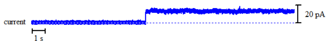
Figure A2 - 120: Above: bilayer activity of 13 with Na + ions upon the addition of 25 \mu l stock solution of 13 in DMSO. Right: histogram displaying the average currents for the above trace: peak 1 = 0.7334 \pm 0.0059 pA and peak 2 = 13.37 \pm 0.0096 pA.
