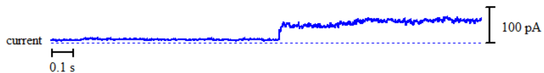
Figure A2 - 125: Above: bilayer activity of 13 with \text{Na}^+ ions upon the addition of 200 \mu\text{l} stock solution of 13 in DMSO. Right: histogram displaying the average currents for the above trace: peak 1 = 9.247 \pm 0.0034 pA, peak 2 = 48.57 \pm 0.5281 pA and peak 3 = 66.81 \pm 0.1317 pA.
