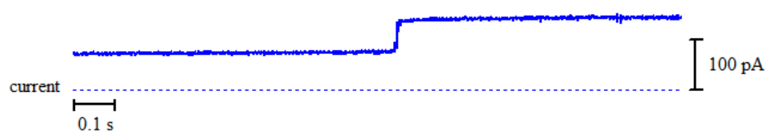
Figure A2 - 2: Above: bilayer activity of 8 with Na + ions upon the addition of 100 \mu l stock solution of 8 in DMSO. Right: histogram displaying the average currents for the above trace: peak 1 = 74.5000 \pm 0.0319 pA and peak 2 = 143.7000 \pm 0.0488 pA.
