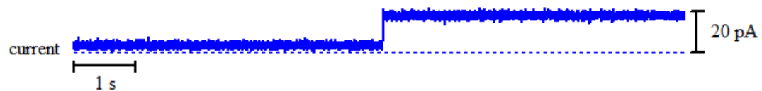
Figure A2 - 137: Above: bilayer activity of 14 with Na + ions upon the addition of 75 μl stock solution of 14 in DMSO. Right: histogram displaying the average currents for the above trace: peak 1 = 3.782 ± 0.0051 pA and peak 2 = 18.43 ± 0.0052 pA.
