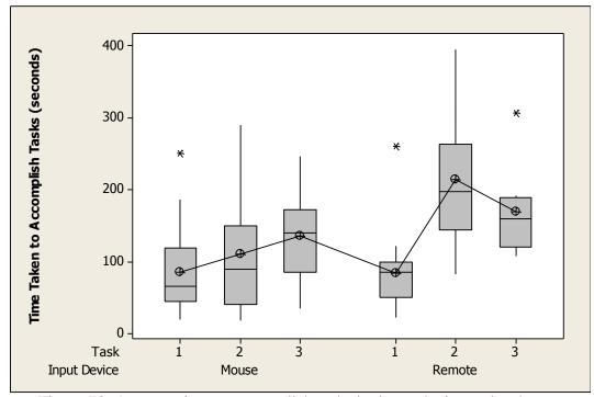
Figure 73. Average time to accomplish tasks by input device and task type
