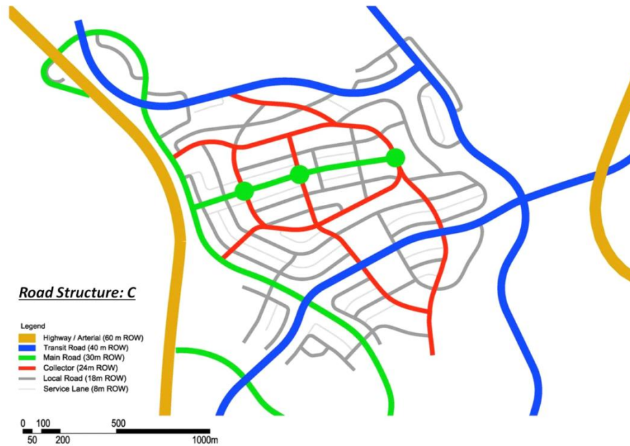
Figure 4.16: Road structure for area C: Southern Gateway, (Sources: GAM, 2010). Modified by the researcher
