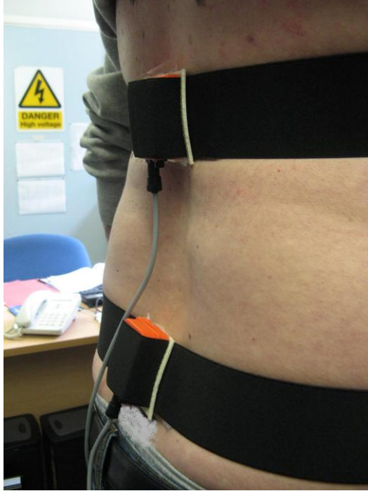
Figure 7.3.1: Attachment of inertial sensors (Xsens) to L1 and S1 spinous processes of participants
