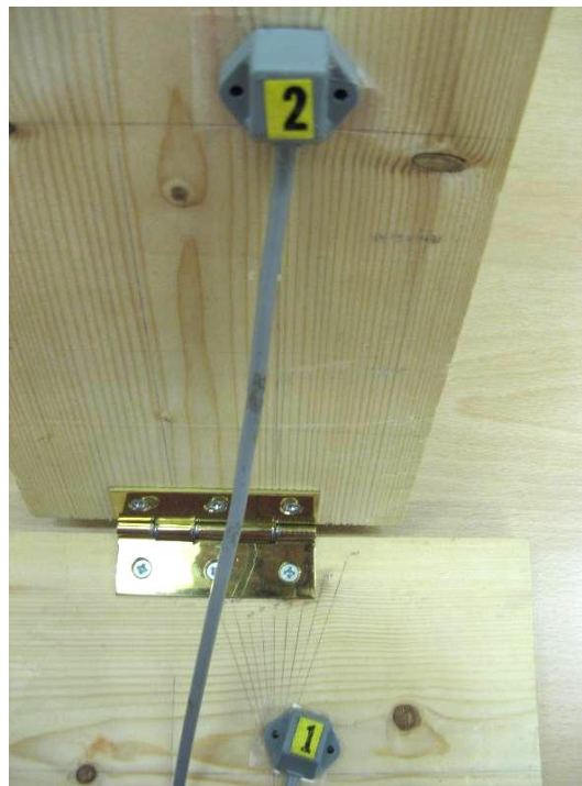
Figure 5.2.3: Configuration 2, the reference sensor was 15° misaligned with the wooden hinged joint movement plane
