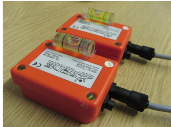
Figure 4.4.2: the Z axis points down on a vertical axis, while X and Y axes are horizontal, spirit levels were used to ensure the alignment to the horizontal axis
