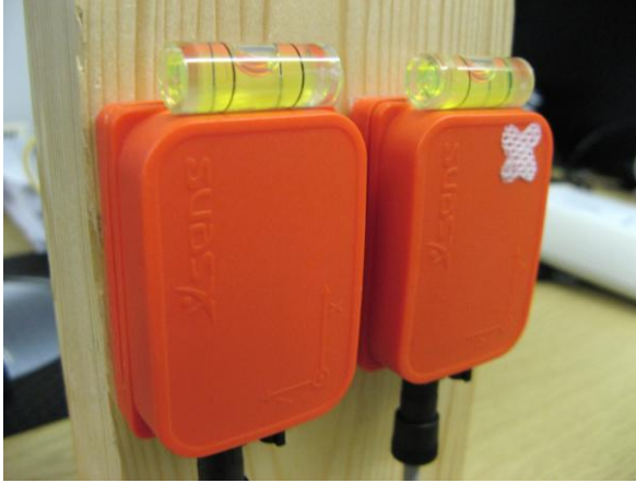
Figure 4.4.3: the X axis points up on a vertical axis, while Y and Z axes are horizontal, spirit levels were used to ensure the alignment to the horizontal axis
