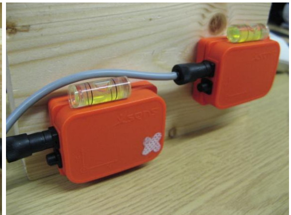
Figure 4.4.6: the Y axis points down on a vertical axis, while X and Z axes are horizontal, spirit levels were used to ensure the alignment to the horizontal axis
