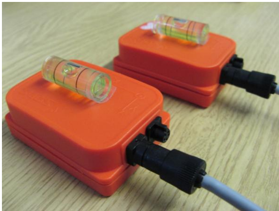
Figure 4.4.1: the Z axis points up on a vertical axis, while X and Y axes are horizontal, spirit levels were used to ensure the alignment to the horizontal axis
