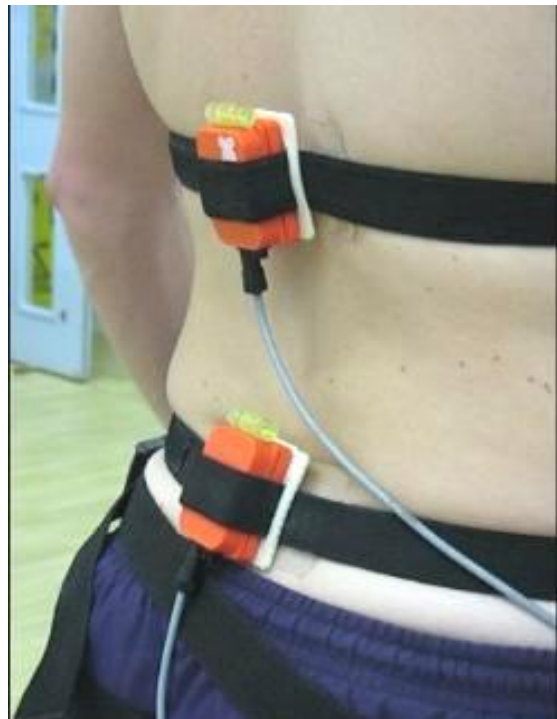
Figure 6.3.3: Attachment of Xsens sensors to the L1-S1 spinous processes
