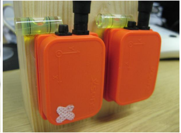
Figure 4.4.4: X axis points down on a vertical axis, while Y and Z axes are horizontal, spirit levels were used to ensure the alignment to the horizontal axis
