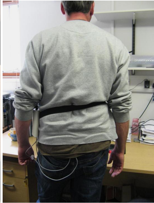
Figure 7.3.2: Sensors stayed underneath clothing and data logger was worn over clothing
