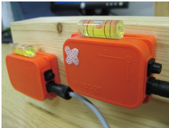
Figure 4.4.5: the Y axis points up on a vertical axis, while X and Z axes are horizontal, spirit levels were used to ensure the alignment to the horizontal axis
