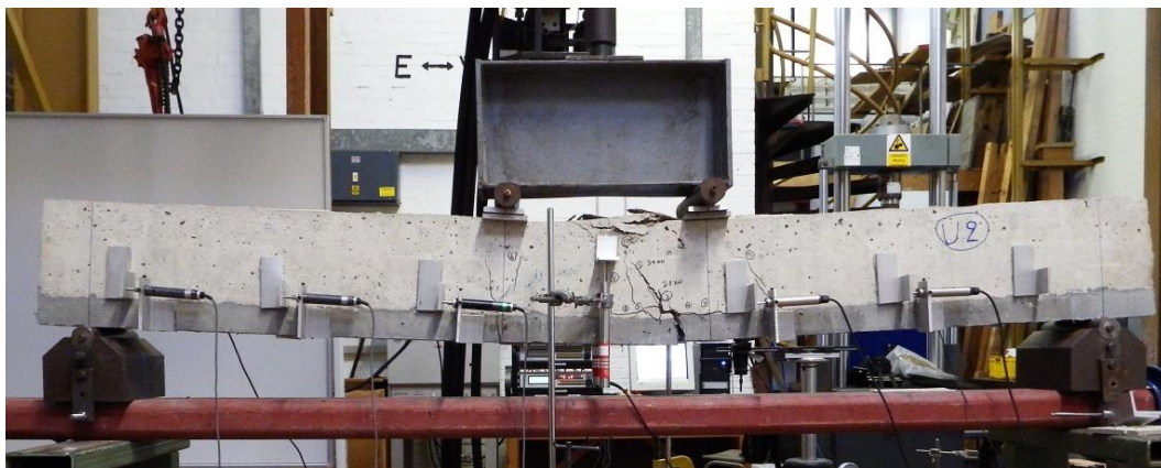
Figure 4.45 Testing of beam UB2: a) appearance of the first cracks, b) propagation of the cracks and c) failure on the compressive side and starting of failure on the UHPFRC layer
