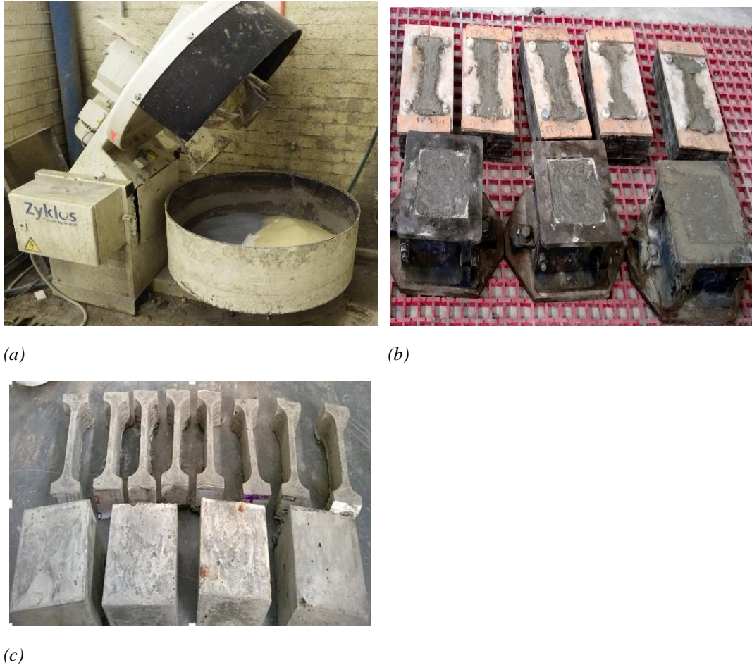
Figure 3.1 Preparation of the specimens: a) mixer used for the mixing the materials b) dog bone shaped and cube specimens after casting c) dog bone shaped and cube specimens after demolding
