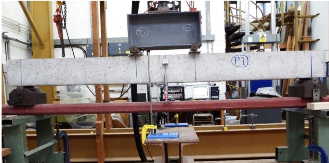
Figure 4.18 Experimental setup for the four point loading tests: a) distance between the two loading points and the span length and b) experimental setup for the control beams
