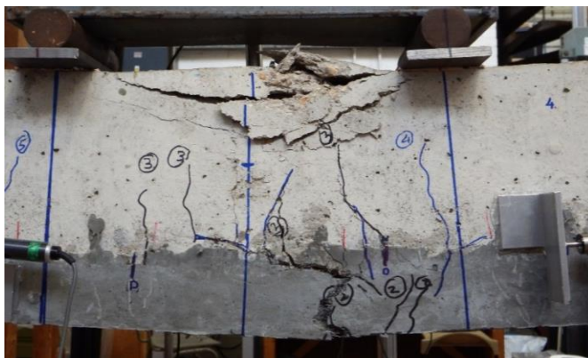
Figure 4.38 Different phases during the testing of beam D2: a) appearance of the cracks, b) the failure of beam on both the compressive and tensile sides and c) beam at the end of the test
