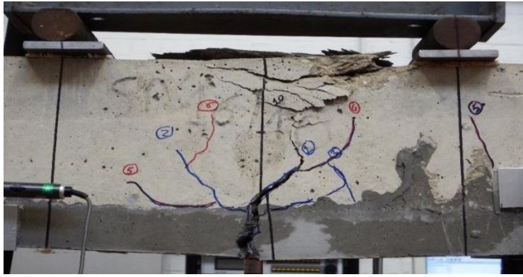
Figure 4.35 Different phases during the testing of beam D1: a) appearance of the first cracks, b) failure of beam on both the compressive and tensile sides and c) beam at the end of the test
