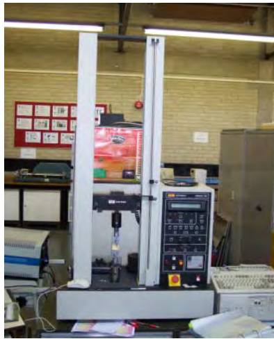
Figure 48 Instron computerised tensile test machine used for dynamic friction tests (original in colour).
