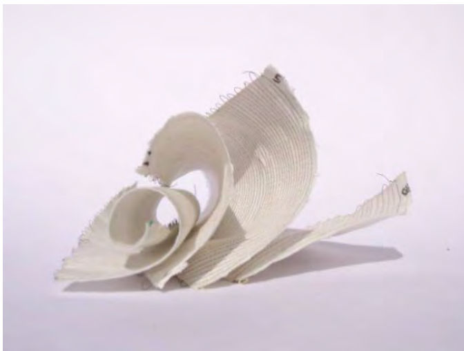
Figure 52 Effect the woven structure can have on the transfer of shape from similarly trained NiTi wires (original in colour).
