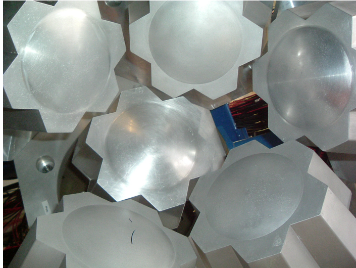
Figure 3.14: A photograph of one of the hemispheres of the RISING array showing the cluster structure, each consisting of seven hexagonal high purity germanium crystals.
