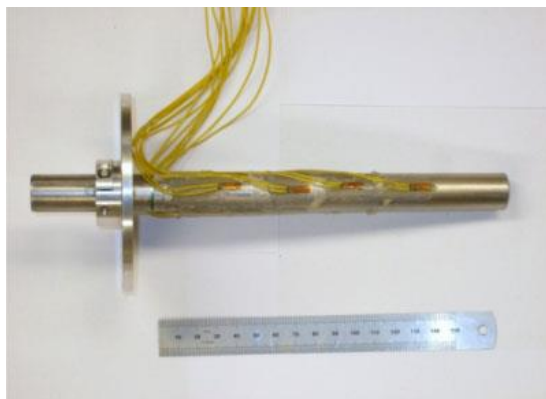
Figure 2. Model hybrid monopile foundation
