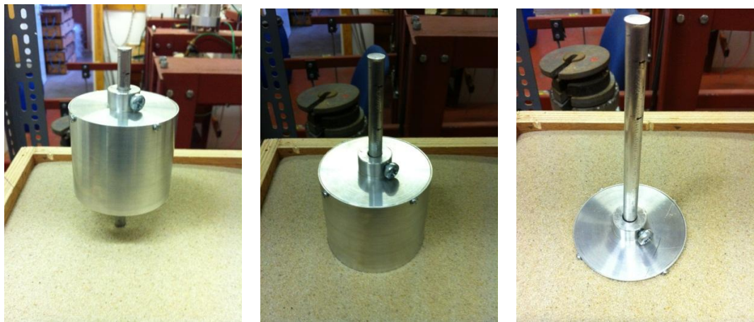
Figure 3.6. Installation of skirted footings following the completion of pile driving
