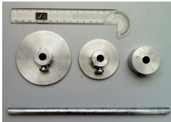
Figure 2. Model foundation system
