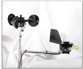
Figure 9.3 Anemometer and wind direction vane
