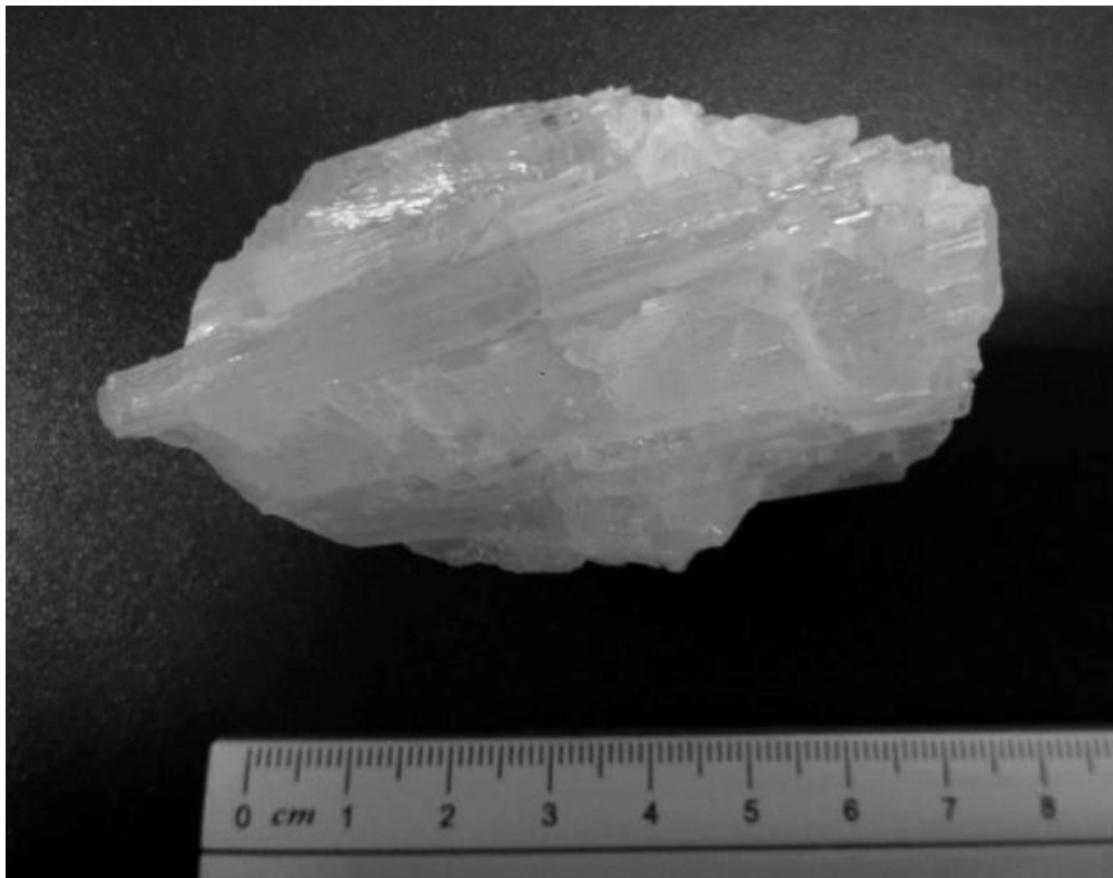
Figure 3.1: Calcite sample (Iceland Spar, Beachy Head) prior to milling.
