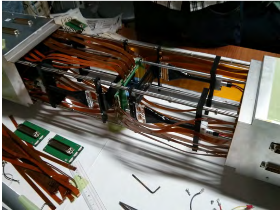
(a) Inside the WAS3ABi chamber. The central structures with ribbon cables attached are the 5 DSSSDs and the plastic scintillators are the black sheets at either side of the DSSSD.
