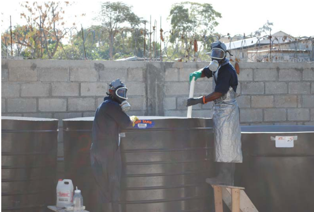
Figure 3.8: Slow mixing phase for the low-pH treatment.
