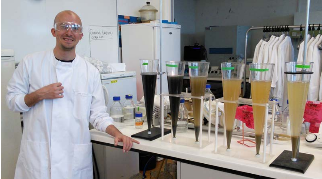
Figure 3.15: Final result of gravimetric test for the measurement of settleable solids
