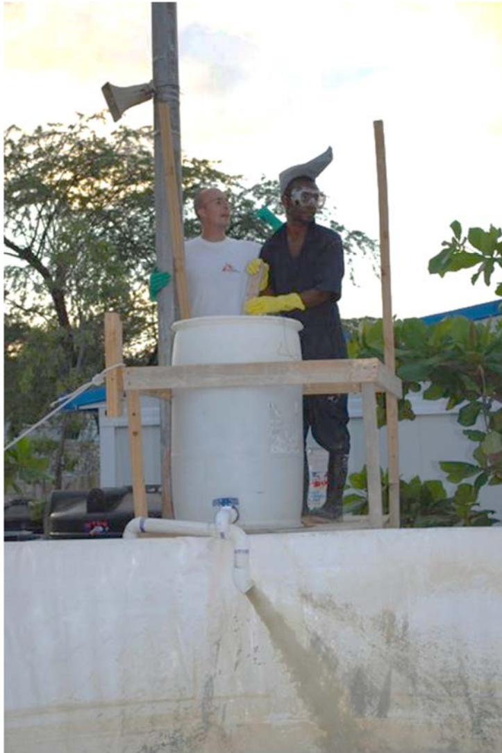
Figure 3.6: Lime slurry preparation: mixed lime slurry was added continuously to the contents of the sedimentation tank in order to approximate a rapid-mixing regime. The inflow hose was positioned to run parallel to the tank wall by means of an 'elbow-joint'
