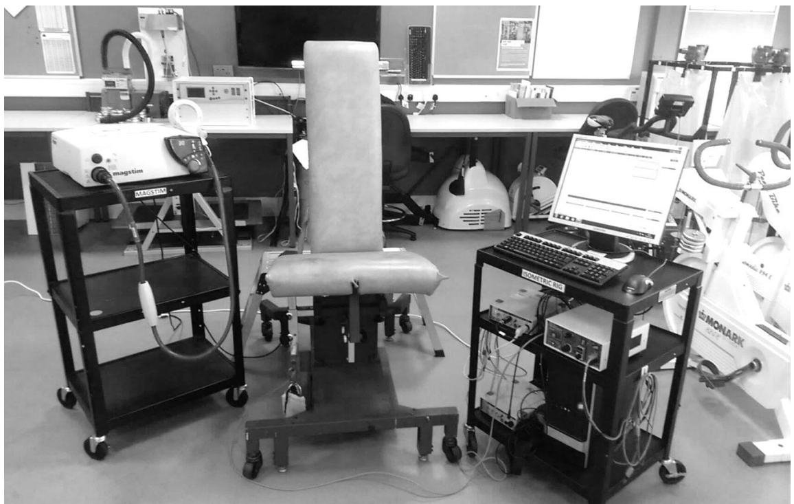
Figure 3.3 The custom-modified and adjustable isometric dynamometer and related equipment at the Welkin Laboratories, University of Brighton.
