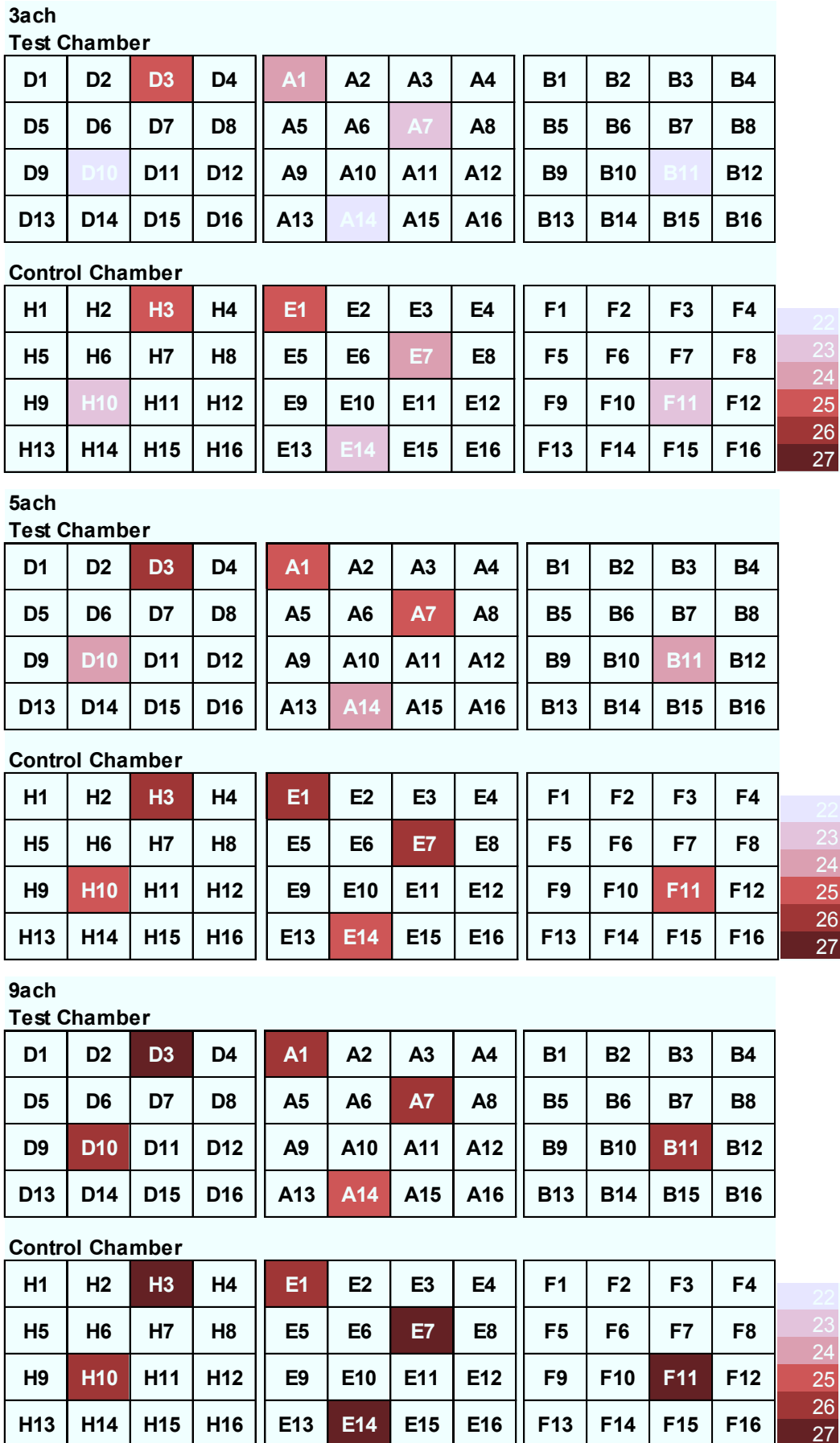
Figure 8.15 Surface temperature distribution in Environmental Chambers after 10 hours
