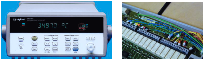
Figure 8.6 The Agilent Benchlink data logger with multiplexer card (showing wiring of air temperature probes)
