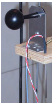
Figure 8.5 Room temperature sensor (black globe) and an air temperature probe
