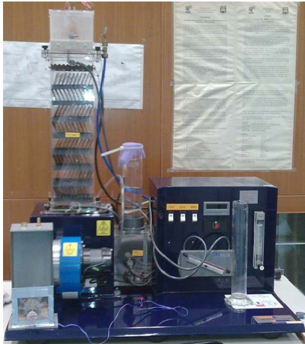
Figure 3. Cooling tower experiment unit
