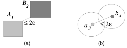
Fig. 5. Qualified combinations for the join. (a) Nonleaf combination. (b) Leaf combination.
