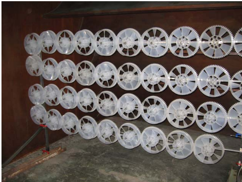
Figure 5-9 Wind tunnel test of micro wind turbine system.
