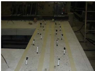
(a) Inserted FRP anchors and prepared concrete surface
