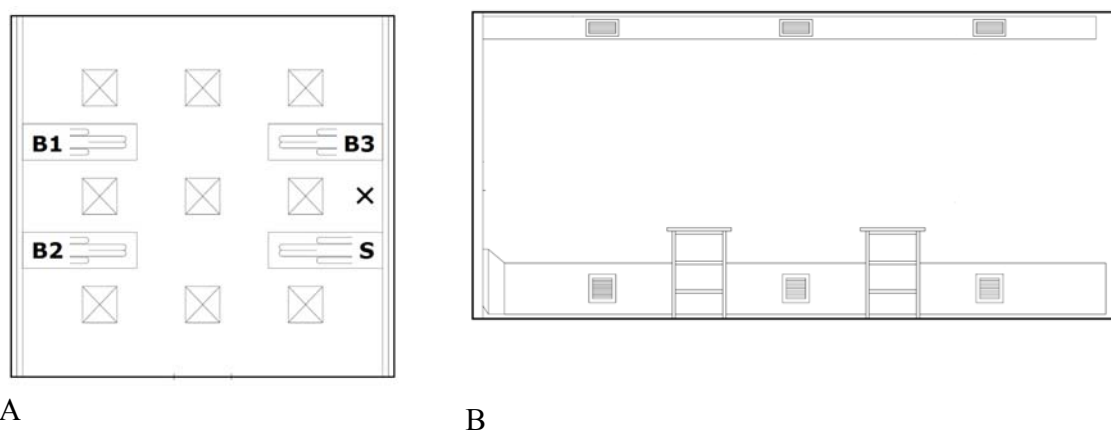
Figure 1. Test room at University of Hong Kong. The horizontal section, Figure 1A, shows the distribution of the nine diffusers and the four beds. One bed indicates the location of the source manikin, and the other beds show the location of the target manikins. The exhaust openings consist of either six openings close to the ceiling or six openings close to the floor, Figure 1B.
