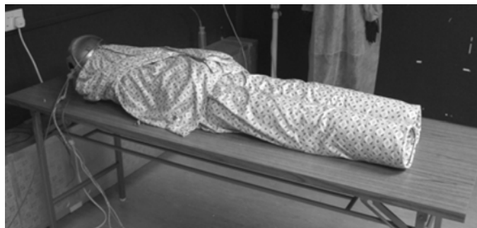
Figure 3. Thermal manikin lying on a bed in the full-scale hospital ward.
