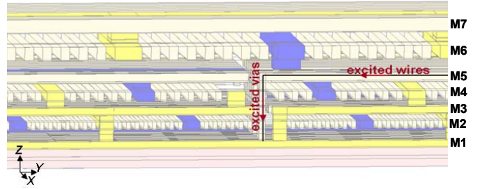
Fig. 4. Zoomed in view of a 45 nm technology backend structure. The monitored V_{DD} wire is from x = 0 \mu\text{m} , y = -125 to 125 \mu\text{m} , z = 1.296 \mu\text{m} . The monitored S4 wire is from x = 0.938 \mu\text{m} , y = -125 to 125 \mu\text{m} , z = 1.296 \mu\text{m}
