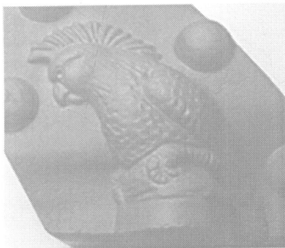
Figure 4. A prototype of a parrot insert with textured free-form surface
