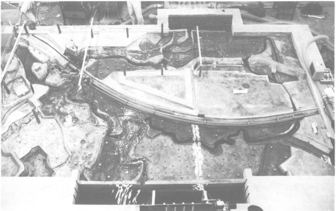
Fig. 2 Partial flooding of low lying areas caused by a 1 in 2 year flood
