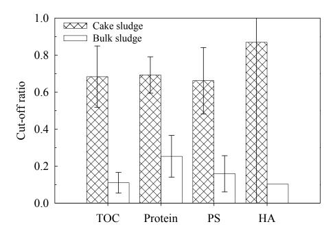
Fig. 5. Cut-off ratios by the 0.4-µm filter for the organic materials and their components in the supernatants of the bulk sludge and the resuspended cake sludge.
