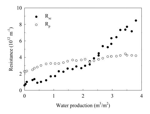
Fig. 1. Sludge cake resistance and pore fouling resistance determined for a typical test run of the SMBR with a sludge concentration of 6 g SS/L, an effluent flux of 0.3  $\text{m}^3/\text{m}^2\cdot\text{d}$  and an aeration intensity of 10 L/m<sup>2</sup>·s.
