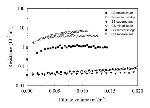
Fig. 2. Comparison of the bulk sludge and the resuspended cake sludge for the filterability of the mixed sludge liquor and its settled sludge and supernatant.
