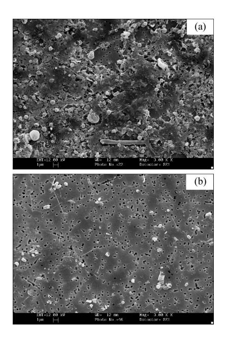
Fig. 6. SEM micrographs of the organic materials that were retained on the filters from the supernatants of (a) the resuspended cake sludge and (b) the bulk sludge.
