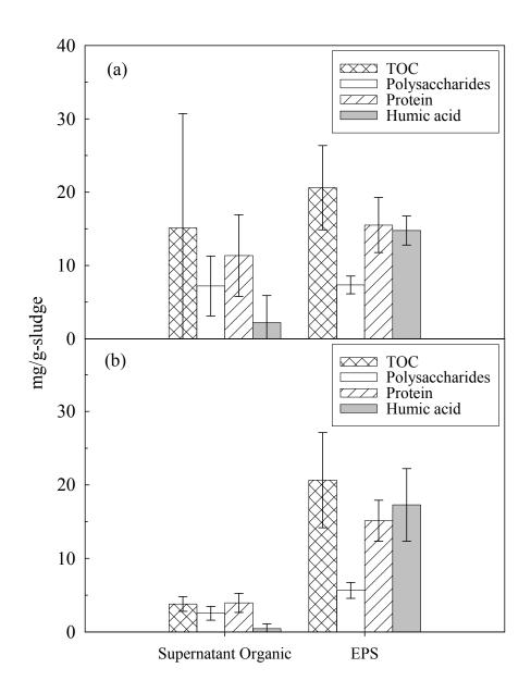
Fig. 4. Organic materials and their composition in the supernatant and the EPS of (a) the cake sludge removed from membrane and (b) the bulk sludge of the SMBR suspension.
