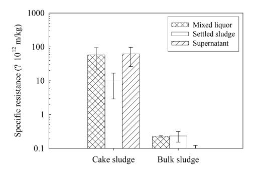
Fig. 3. Specific resistances of the cake sludge that was removed from the membrane and the bulk sludge of the SMBR suspension.
