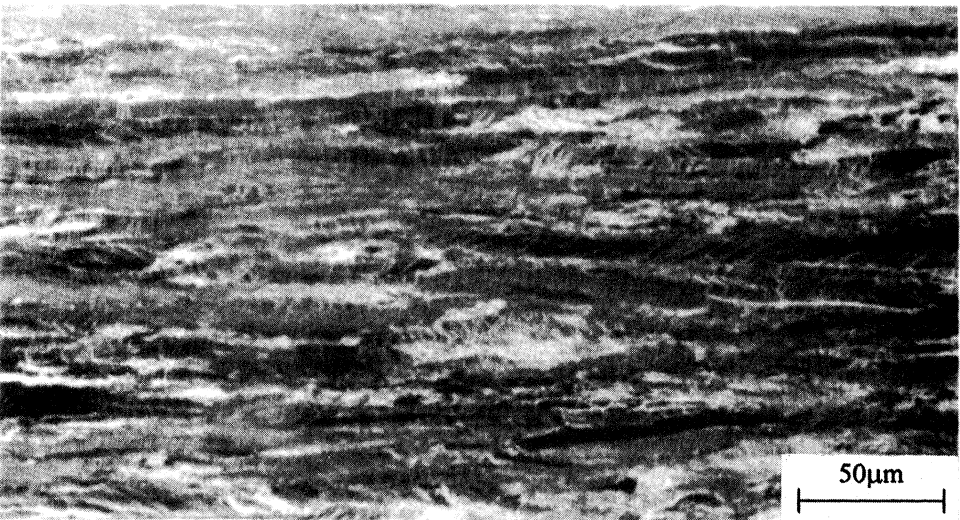
Figure 5 (c) Crystallographically etched microstructures of copper rolled to 75% reduction in a single pass at 500°C.
