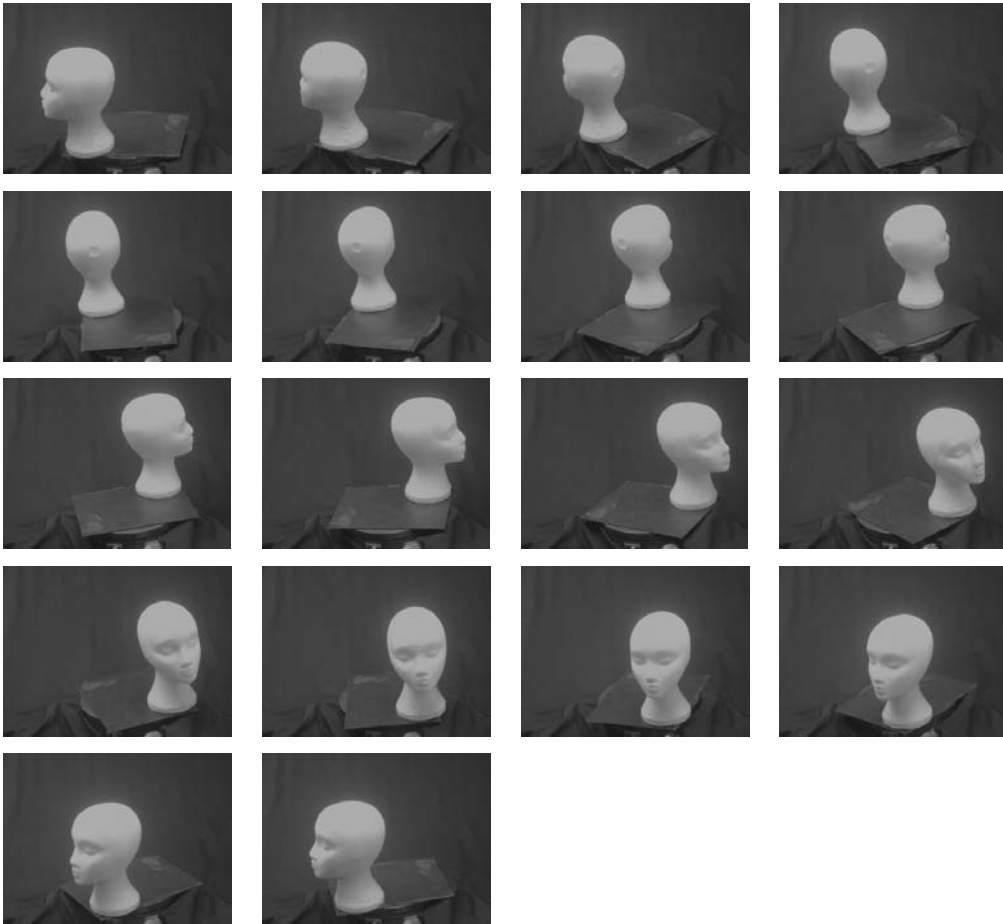
Fig. 5. Eighteen images of a polystyrene head model under controlled circular motion. Each image was taken after rotating the model by 20^\circ on a turntable with a resolution of 0.01^\circ .
