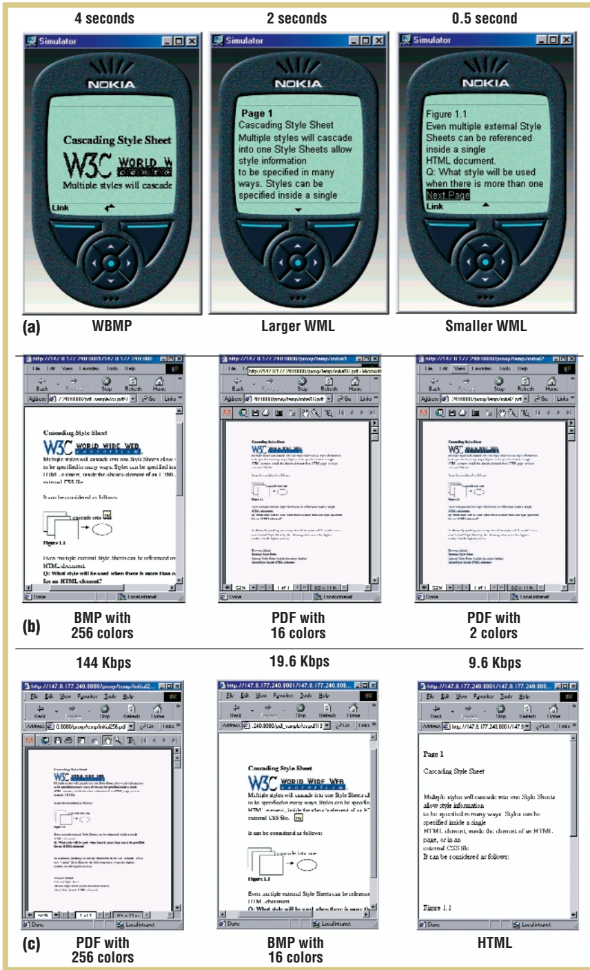
Figure 7. The content adaptation system adjusts the content version to meet changing requirements: (a) maximum tolerable downloading time; (b) color depth preferences; (c) available bandwidth.
