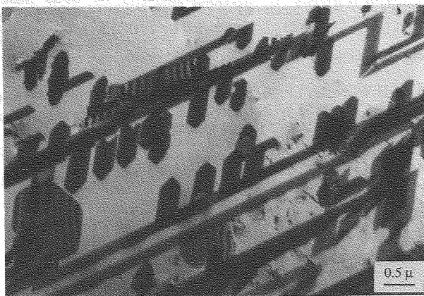
Fig. 5 - TEM micrograph of a thick area showing stacking fault overlapping after in-situ annealing at 780°C.
