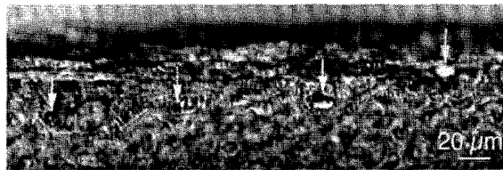
Fig. 3. Cross-sectional view of a series of cavities made in the bulk of skin with 100-fs, 20- \mu J pulses. Each pulse was focused at a different depth relative to the skin surface.
