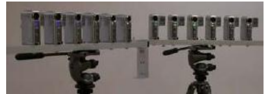
Fig. 6. Configuration of our multiple video cameras system.
