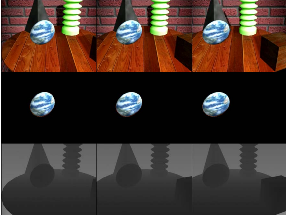
Fig. 1. Snapshots of (Top) synthetic PV “synthesis”; (Middle) the IBR object “ball”; (Bottom) the depth maps of the synthetic PV “synthesis”.
