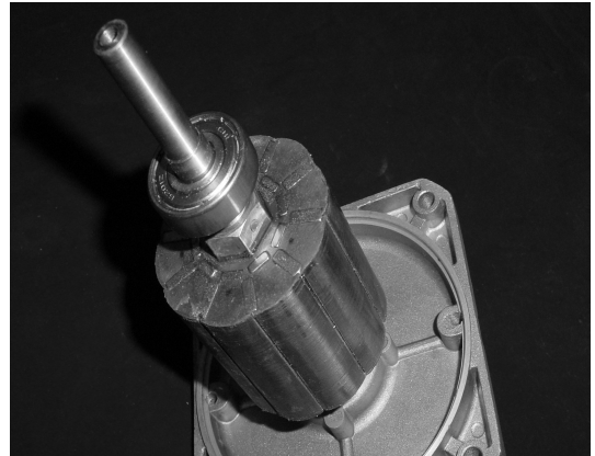
Figure 10. Rotor of the proposed IPMSM.
